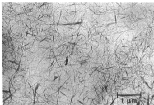
FIGURE 15 TEM-picture of microfibrillar cellulose. Dissolving pulp softwood, hydrolysis in 2.5 M HCl at 105°C for 1 h, thereafter 10 passages through the slit homogenizer. Philips EM 400, magnification 10.000 x. Uranium acetate shadowing. Black line 1 μm.
